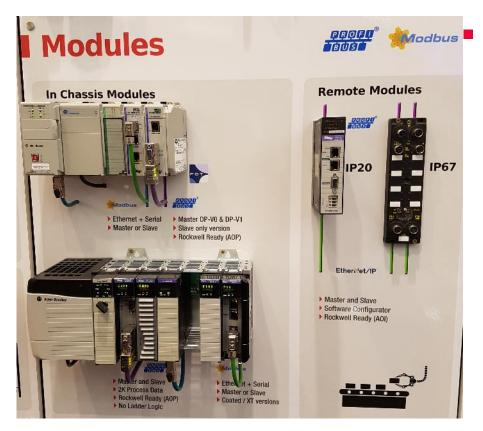
For CompactLogix and ControlLogix
