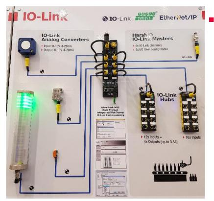
All-In-One: Digital + Analog IO signals + I/O hub to simplify Ethernet Infrastructure
