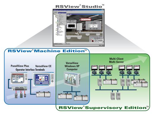
Rockwell Automation Visualization Solutions combine dedicated and open hardware platforms with RSView Enterprise Series software for machine level and supervisory level HMI.
